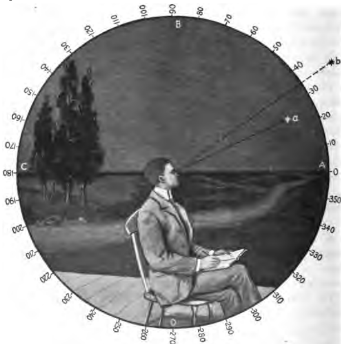
FIG. 3.—Showing the angle between two stars, a and b , as seen by an observer. In the figure this angle is about 10^{\circ} . The figure also shows how degrees are counted round the circle, passing from the line going horizontally to the right. A right angle, or 90^{\circ} , measures from the horizon A to the zenith B . Two right angles, or 180^{\circ} , bring us to the horizon on the left; the third right angle, making 270^{\circ} , takes us to the point D below, and the fourth one will carry us round to A , where we started.
